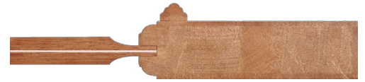
Section view of a Legacy panel and stile door with Legacy raised molding.
